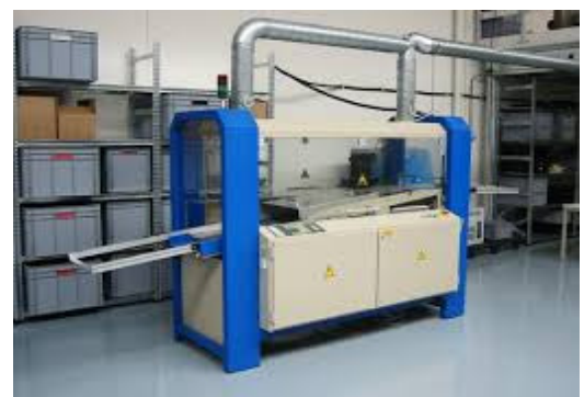
wave soldering machine fume extraction
