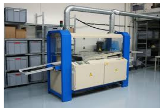
wave soldering machine fume extraction
