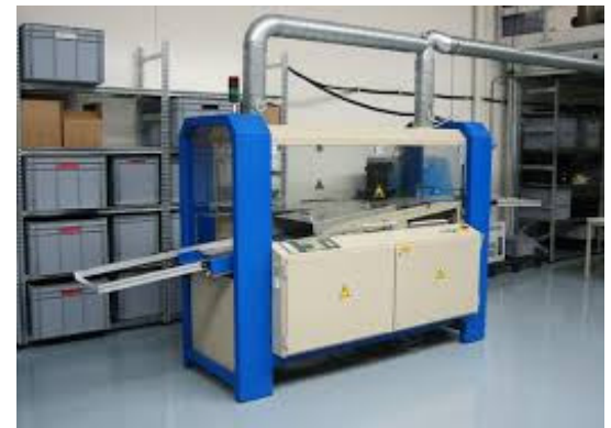
wave soldering machine fume extraction
