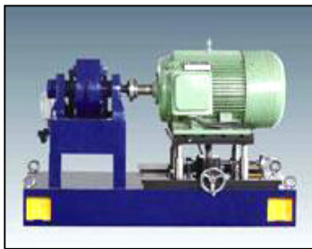
Dynamometer Test Bench (Diesel Engine)
