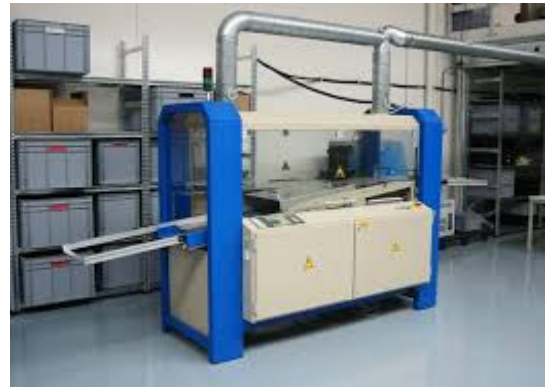
wave soldering machine fume extraction
